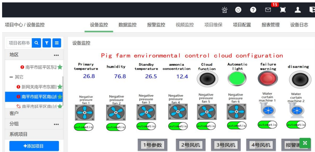
Figure 2. Human-Machine Interface for Pig House Environmental Control System.
